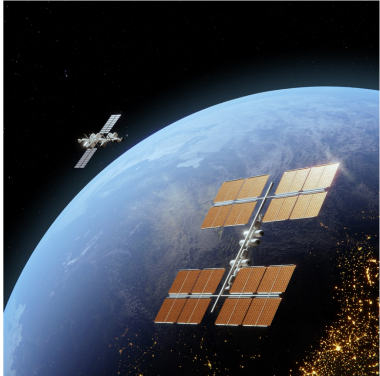
Space station with next generation, 50-kilowatt class solar array wings. Solestial's silicon solar blanket technology will allow for arrays larger than any ever built, while also maintaining lower mass and competitive efficiency. The array will be developed in collaboration with Opterus Research & Development ("Opterus") and will integrate Solestial solar blankets with Opterus' patent pending Retractable-Rollable Mast Array ("R-ROMA") advanced deployable solar array structure.
